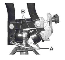
2. Place the circlip (a) over the tow ball of the vehicle. Place the two pieces (b) either side of the ball of the car.
