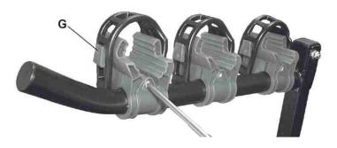
Insert the adjustable holders for the bicycles frames (g) onto the arms and tighten with a screwdriver Install the bicycle and secure it with the retainers (g)
