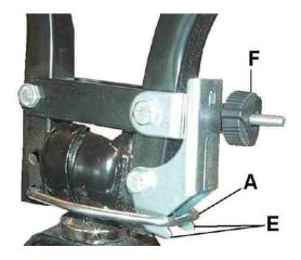
4. Lock the handle by inserting the safety pin (d) into the hole in the handle (c) Place the ring (a) in the hooks (e) and tighten the thread (f) in a clockwise direction.
